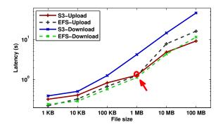
Fig. 4. Average upload/download latencies for files in different sizes to/from S3 and EFS.
