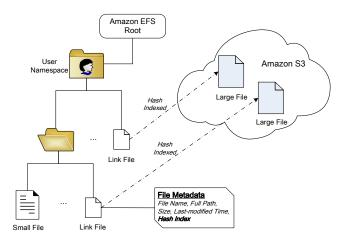
Fig. 2. The hybrid system design using the intuitive approach (large files stored in S3 are indexed by link files).
