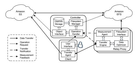
Fig. 6. System framework of HyCloud (including interaction among components and their internal module calls).
