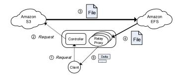
Fig. 1. Architectural overview of HyCloud, and a typical process for a client to download a large file from the hybrid cloud storage services.
